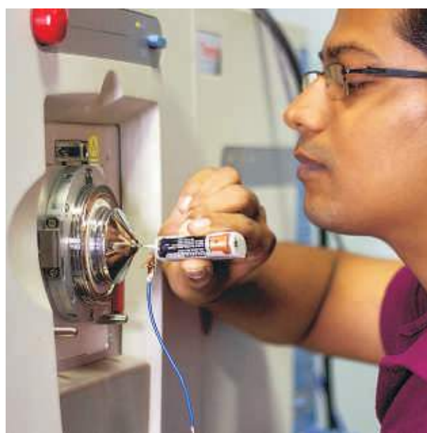
A) Schematic representation of the ionization process from CNT paper. B) Photograph of the ionization source showing paper triangle and battery along with a grounding electrical connection. C) Mass spectra of triphenylphosphine (M) at 3 kV, 3 V, and 1 V from wet CNT paper. D) Field emission scanning electron microscopy (FESEM) image of CNT-coated paper. E) Isotope distribution of the protonated molecule at 3 V. F) MS2 spectrum of the parent ion at m/z 263.
