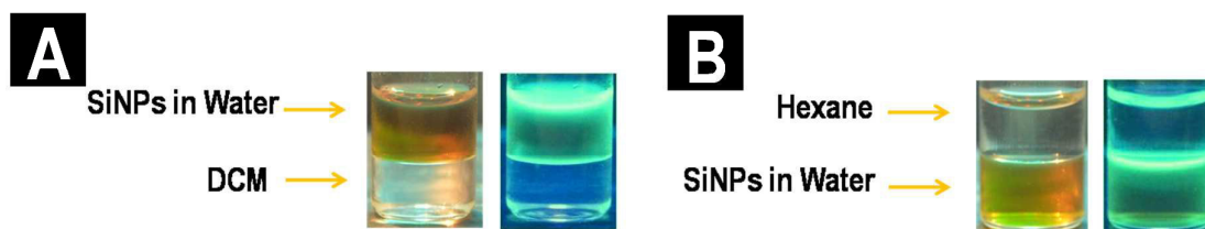
Figure S13. (A) & (B) shows the excellent hydrophilic nature of the as-prepared Si NPs where organic solvents having different densities i.e. DCM and Hexane were used to check its miscibility with water dispersible Si NPs.
