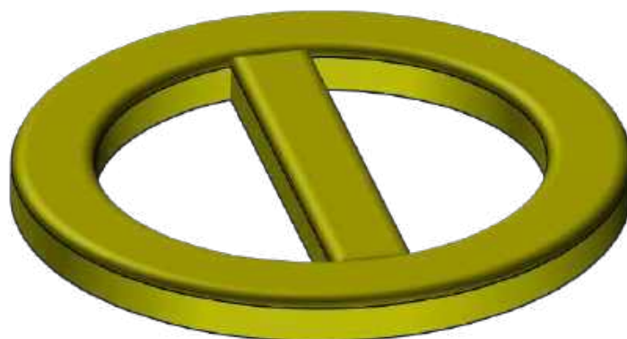
Figure S1. Schematic image of a laser cut mesh from brass foil that was used for interfacial thickness measurement.
