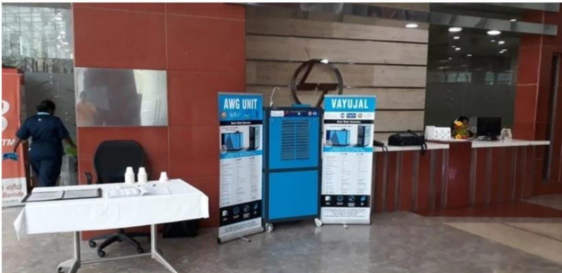
The machines tap potable water using humidity from the atmosphere. Express Photo: Vayujal
