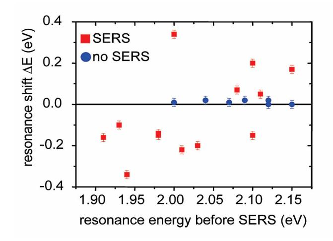
**Figure 5.** Shift of the longitudinal-mode Rayleigh scattering resonance energy  $\Delta E$  vs initial resonance energy.
