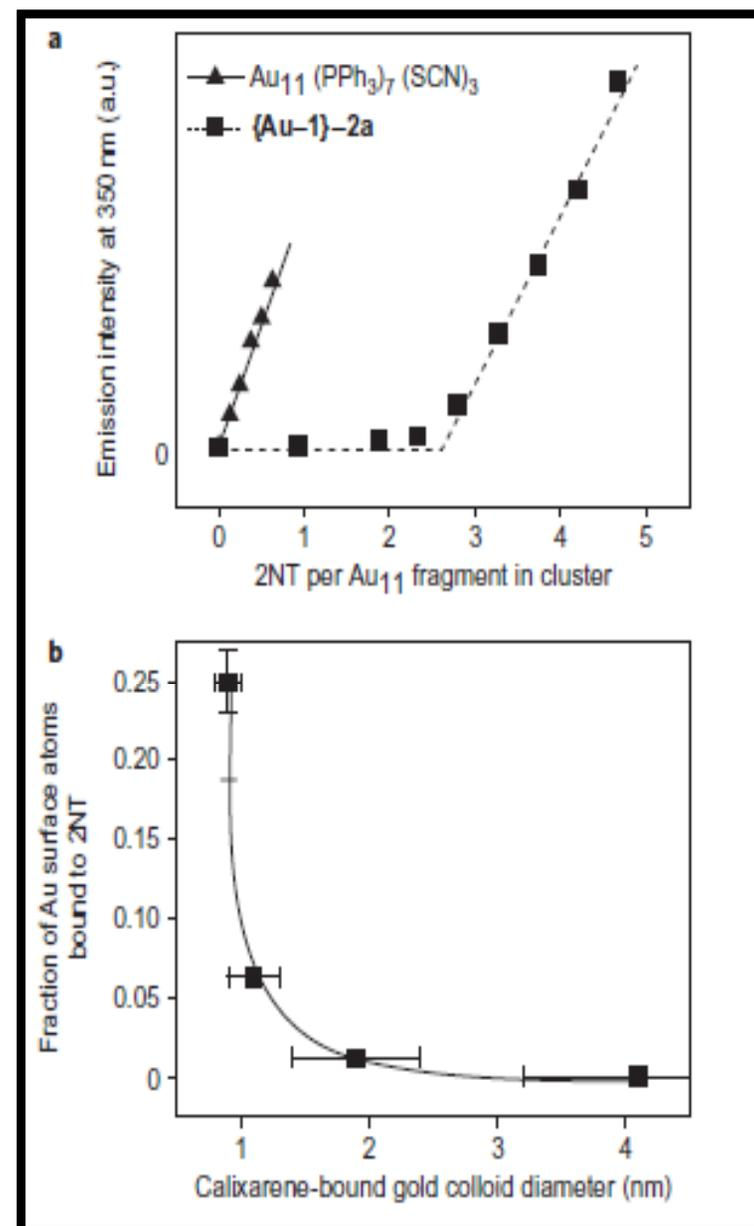
b) Fraction of gold surface atoms that are bound with 2NT (lower  $k$  cluster diameter)
