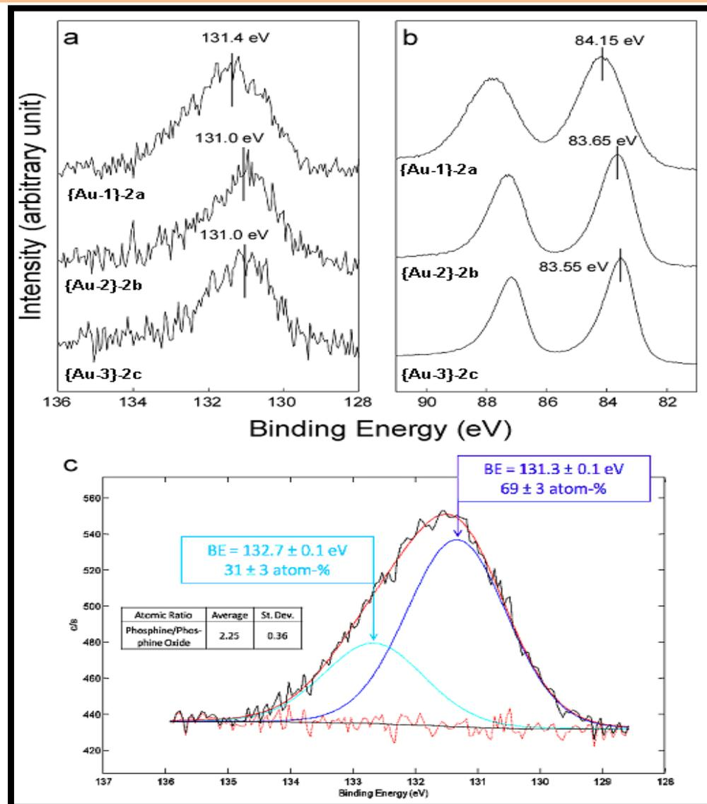
*(a) P 2p and (b) Au 4f XPS results of {Au-1}-2a, {Au-2}-2b, and {Au-3}-2c. Deconvolution of {Au-1}-2a P 2p results in (c) is shown in (c). Binding energy is corrected by C 1s at 2 $\xi$*
