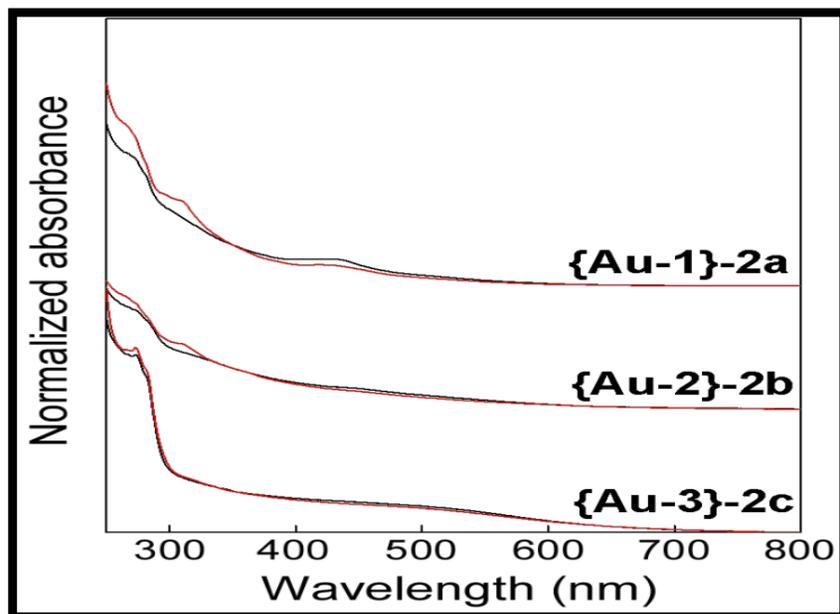
*UV-Vis spectra of gold clusters before (black) and after (red) addition of 40-fold excess 2NT*
