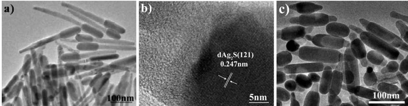
(a) TEM image of rodlike  $\text{Ag}_2\text{S-AgInS}_2$  heterostructures with rodlike  $\text{Ag}_2\text{S}$  as source-host reacted at (a)  $150\text{ }^\circ\text{C}$  and (c)  $170\text{ }^\circ\text{C}$ , (b) HRTEM of the interface showing  $\text{AgInS}_2$  grown on the (121) plane of  $\text{Ag}_2\text{S}$ .
