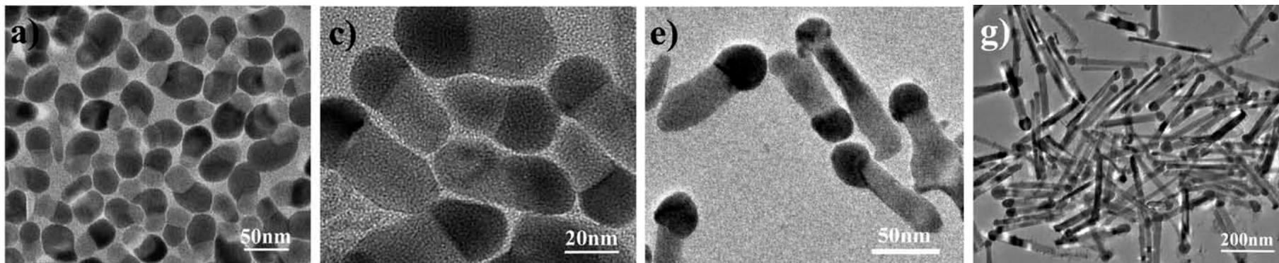
TEM images of Ag<sub>2</sub>S-CdS heterostructures, which show that the length of CdS segment increases with the amount of Cd(dbdc)<sub>2</sub>
