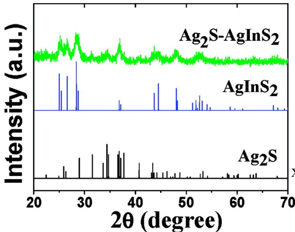
XRD pattern of Ag<sub>2</sub>S –AgInS<sub>2</sub> heterostructure
