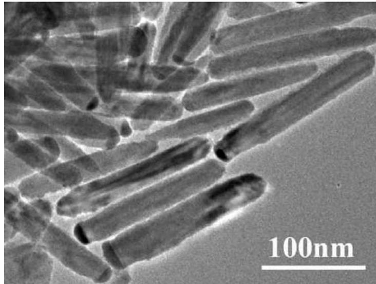
TEM image of the  $\text{AgInS}_2$  nanorods with a small  $\text{Ag}_2\text{S}$  segment
