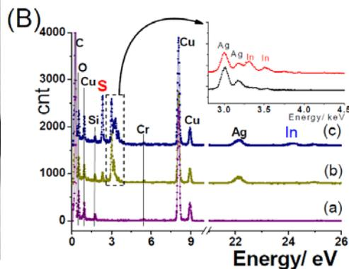
(A) TEM image of  $\text{Ag}_2\text{S}$ - $\text{AgInS}_2$  heterostructured nanocrystals. (B) The EDS spectra recorded (a) on the carbon film for comparison, (b) on the area 1 marked by a circle in A, which shows the existence of Ag and S, and (c) on the area 2 marked by a circle in A, which shows the existence of Ag, In, and S. The EDS spectra recorded on several different heterostructure NC show the same element composition.
