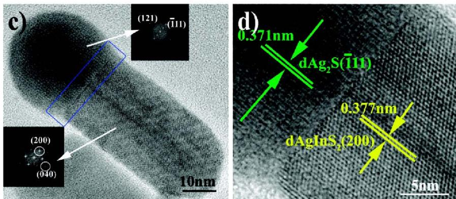
(a) Typical TEM image of the obtained  $\text{Ag}_2\text{S}$ - $\text{AgInS}_2$  heterostructure nanocrystals (b) HRTEM image shows the lattice planes of grain boundary. (c) TEM image of a typical  $\text{Ag}_2\text{S}$ - $\text{AgInS}_2$  heterostructure nanocrystal. The insets show the corresponding FFT, which further gives the detailed structure of the heterojunction. (d) HRTEM image from the area circled by a blue line in (c).
