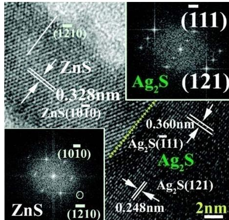
TEM image and EDS spectra of typical synthesized Ag<sub>2</sub>S-ZnS NWs heterostructures
