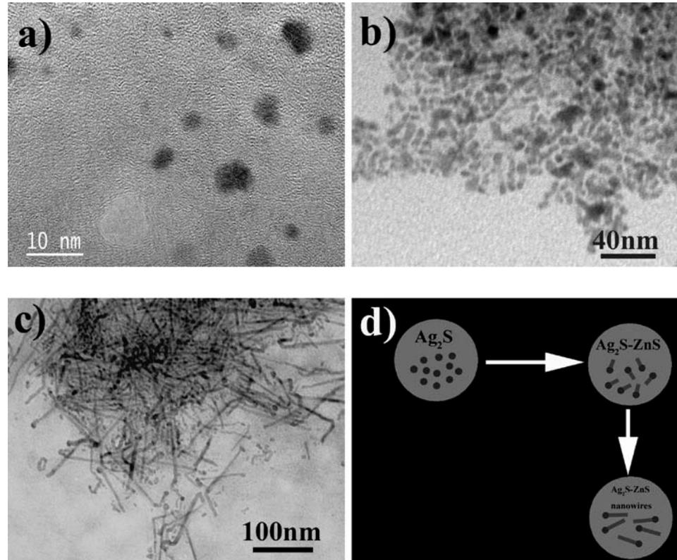
The growth process for the Ag<sub>2</sub>S-ZnS NWs heterostructures at various stages as the temperature increases. TEM images of (a) the Ag<sub>2</sub>S NCs formed when the system was heated to 130 °C, (b) the shorter ZnS nanorods grown on the Ag<sub>2</sub>S NCs when heated to 150 °C, (c) the elongated ZnS NWs with Ag<sub>2</sub>S NCs “head” were formed when further heated to 170 °C. (d) A schematic diagram of the heteroepitaxial growth process of ZnS NWs on Ag<sub>2</sub>S NCs.
