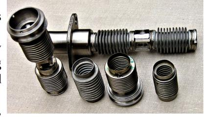
4. Hydroformed and rolled bellows are limited to metals with high plastic elongation characteristics whereas welded bellows may be fabricated from a wider variety of standard and exotic alloys, such as stainless steel and titanium, as well as other high-strength, corrosion-resistant materials.
