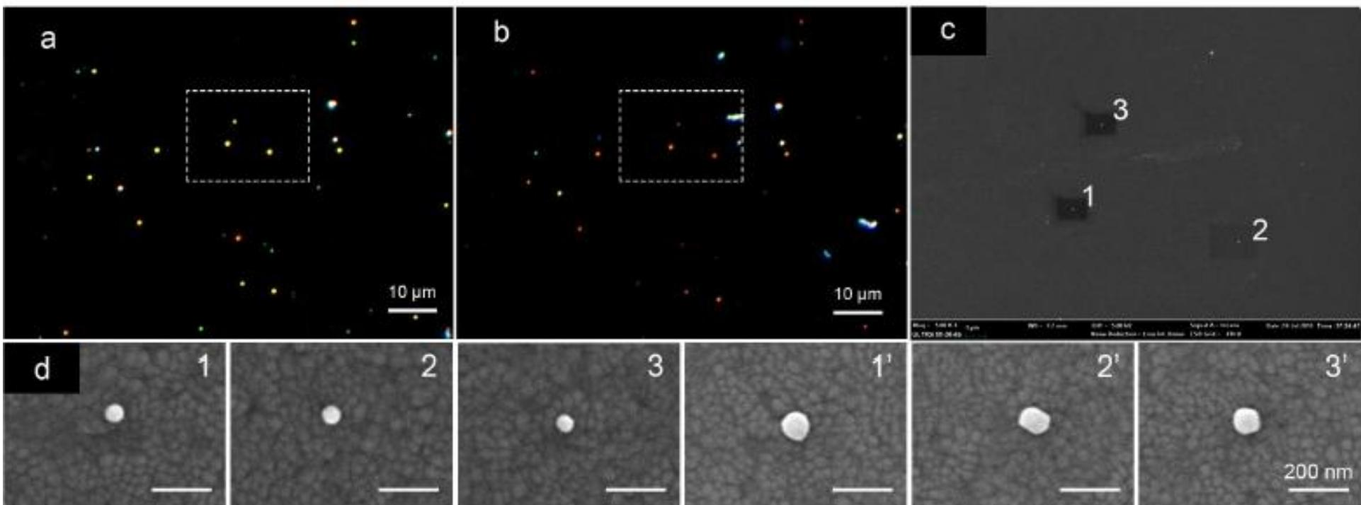
Figure. True color images of GNPs Plasmon resonance Rayleigh scattering before (a) and after (b) the formation of Au@Cu core-shell nanostructure. c, Corresponding SEM image of selected region in a. d, Enlargement SEM images of each single GNP with corresponding number (1~3: original GNPs, 1'~3': Au@Cu NPs). GNPs in 20 μM CuCl<sub>2</sub> containing 25 nM NADH for 3 h.
