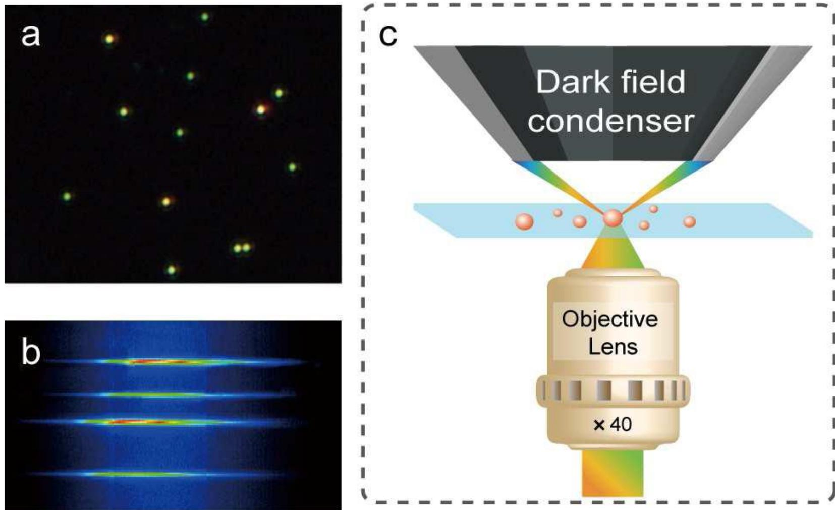
Figure. a, A typical dark-field Rayleigh scattering image of GNPs modified on a microscopy slide; b, Corresponding scattering spectra of single GNPs in slit. c, Detailed experimental configuration.
