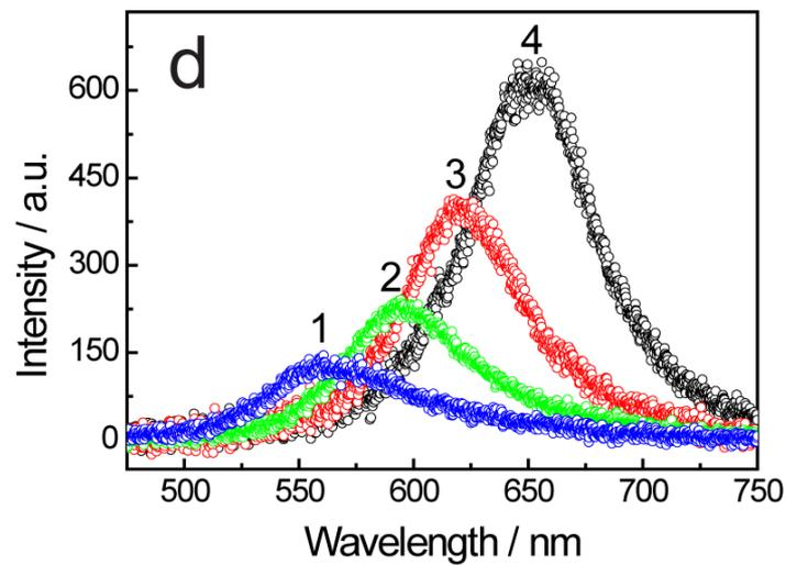
Figure. a, SEM images of 50 nm GNPs. b, UV-vis spectra of seed GNPs and 50 nm GNPs. c, Dark-field color images of GNPs immobilized on microscopy slide. d, Corresponding PRRS spectra of single GNP with different size
