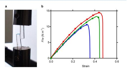
• Joints made of S0.1 gel were stronger than the gel itself and failure occurred outside the bonding junction.
