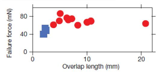
The failure force measured by the lap-shear adhesion test for lap joints of various overlap length. Red circles indicate fracture outside the joint; blue squares indicate interfacial failure by peeling.
