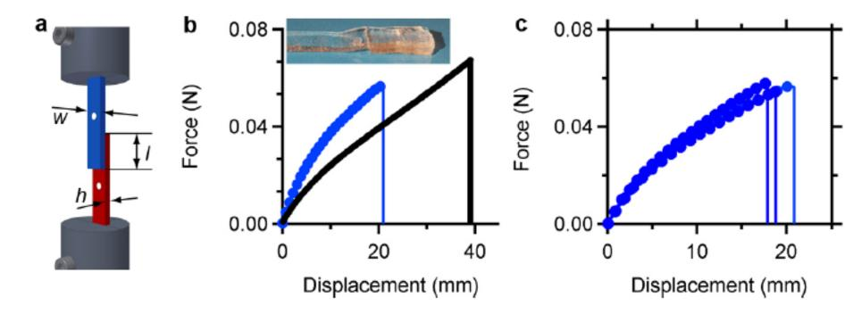
(a) Lap-joint geometry. Displacement was measured by a video extensometer that followed two markers (white dots), which were placed at a distance of 5mm from the edge of the lap joint. The total length of the assembled ribbons was 40mm. w denotes the width and h the thickness of gel ribbons. I is the overlap length.
