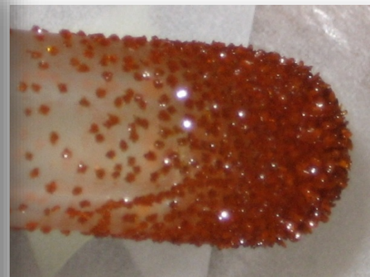
Crystals of ferrocene after purification by vacuum sublimation
