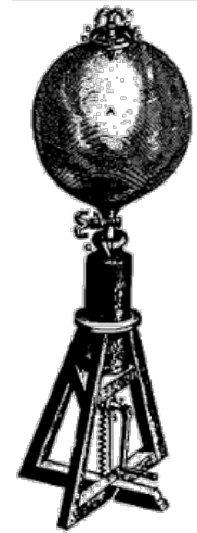
Fig. 3 Piston pump designed by Robert Boyle and built by Robert Hooke in 1658-9.
