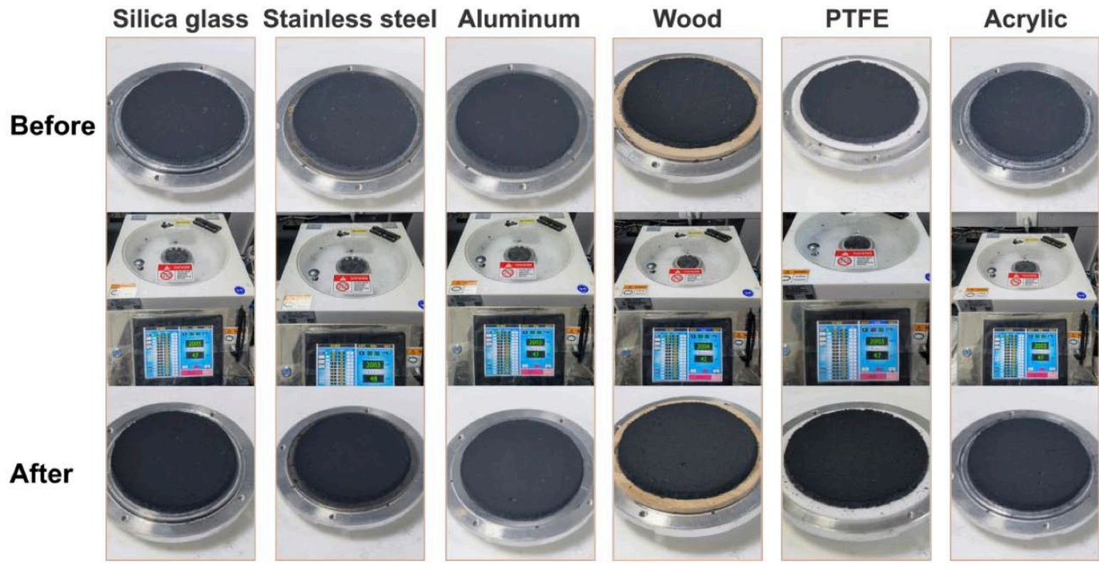
Supplementary Fig. 20 | The adhesion properties of dry HIPG on different substrates containing silica glass, stainless steel, aluminum, wood, PTFE, and acrylic under a rotation speed of 2000 rpm. The dry HIPGs could rotate at a high speed of 2000 rpm for one minute and still tightly adhered to the substrate with no deformation or damage.
