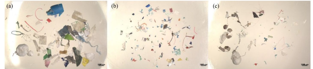
Fig. S3. Photographs of MPs taken under an optical microscope platform: influent (a), aqueous activated sludge (b) and effluent (c).
