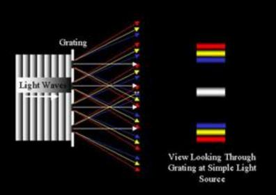
An optical device used to disperse light into a spectrum. It is ruled with closely-spaced, fine, parallel grooves, typically several thousand per cm, that produce interference patterns in a way that separates all the components of the incoming light. A diffraction grating can be used as the main dispersing element in a spectrograph.
