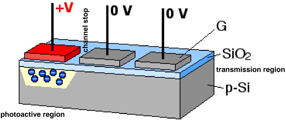
Photoelectric image sensor + shift register
