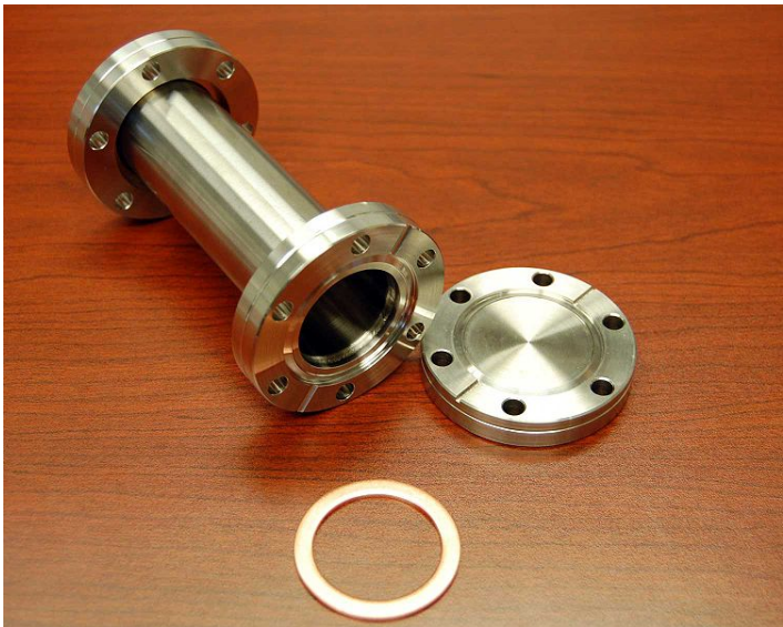
A CF pipe and flange with copper gasket.
