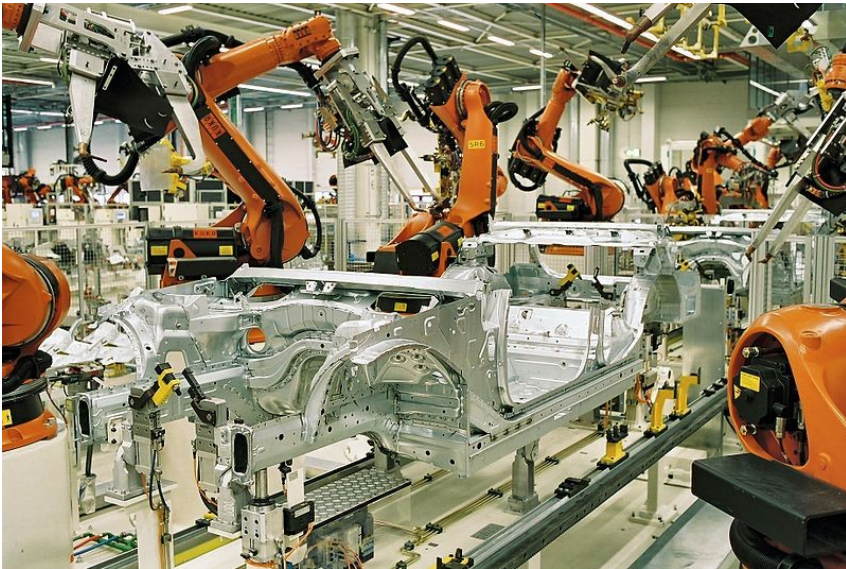
BMW plant in Leipzig, Germany where spot welding robots are used to make car bodies.
