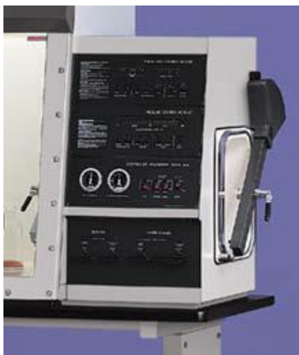
Transfer chamber/ Antechamber
