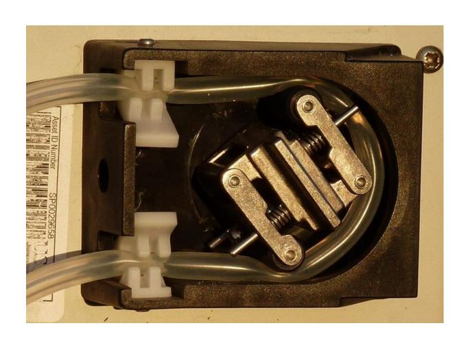
A **peristaltic pump** is a type of positive displacement pump used for pumping a variety of fluids.
