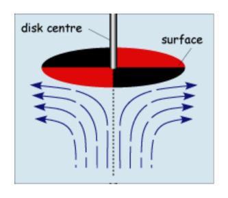
Solution movement caused by rotation of an RDE
