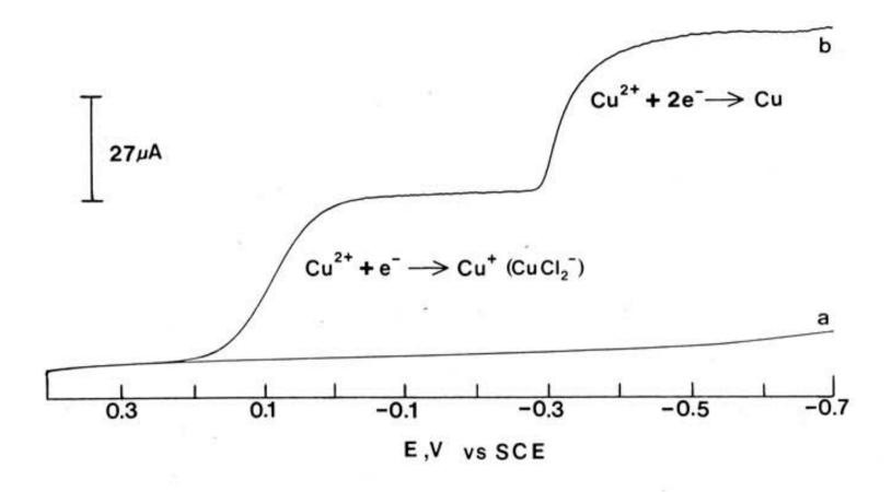
Figure 4. Rotating disk voltammograms of 1 mM  $CuCl_2$  in 0.1 M KCl. Glassy carbon electrode. Scan rate: 100 mV s<sup>-1</sup>. Rotation rate: 1000 rpm. (a) 0.1 M KCl supporting electrolyte. (b) Reduction of  $Cu^{2+}$ .
