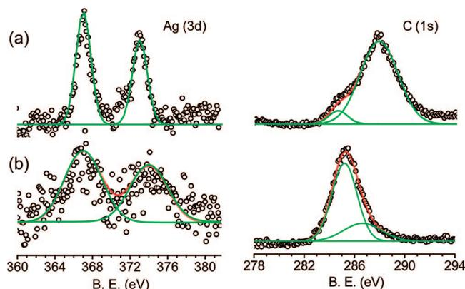
**Figure 2.** Ag(3d) and C(1s) core level spectra of the blend before (a) and after (b) e-beam exposure. The relatively higher spread in data points in (b) is due to poor signal strength as e-beam exposed region was limited to  $3 \times 3 \text{ mm}^2$ .
