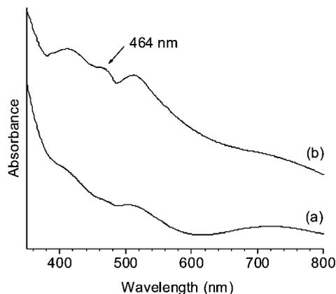
**Figure 3.** Optical absorption spectra of the blend (a) before and (b) after e-dosage. The feature marked with an arrow represents surface plasmon absorption from Ag nanoparticles.
