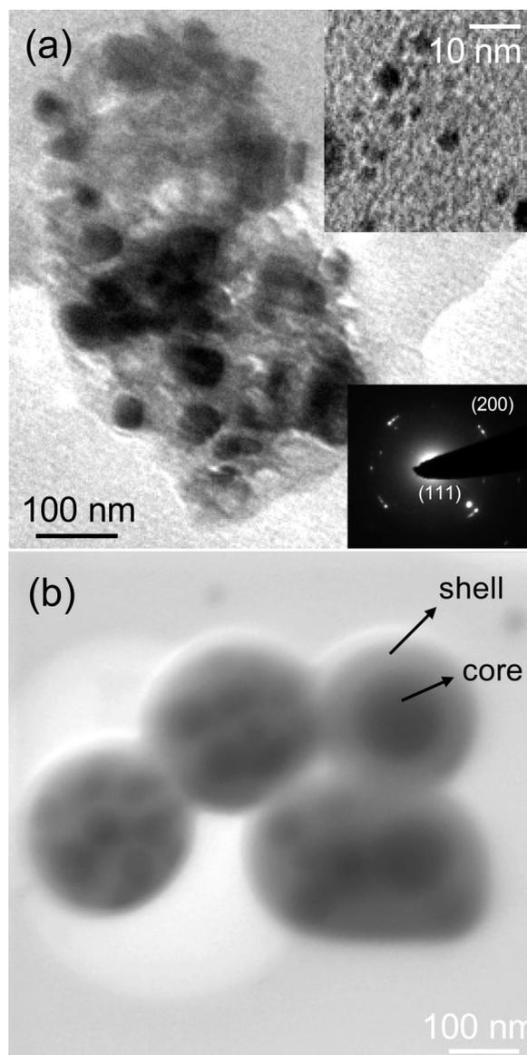
**Figure 4.** (a) TEM image of the e-beam exposed cross-linked blend showing formation Ag nanoparticles. Inset showing high-resolution image (top) and corresponding electron diffraction pattern (bottom). (b) STEM image of the Ag nanoparticle aggregate. The core and shell regions are marked.
