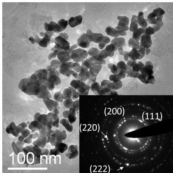
**Figure 5.** TEM image of the e-beam exposed Ag precursor (without polystyrene) showing the formation Ag nanoparticles with the inset containing the corresponding electron diffraction pattern.
