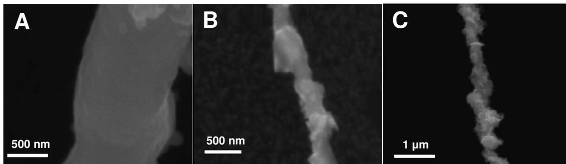
**Figure S3.** SEM images of pristine nickel nanowires synthesized using 80  $\mu\text{L}$  (A), 200  $\mu\text{L}$  (B) and 500  $\mu\text{L}$  of hydrazine hydrate, showing the changes in surface morphology.
