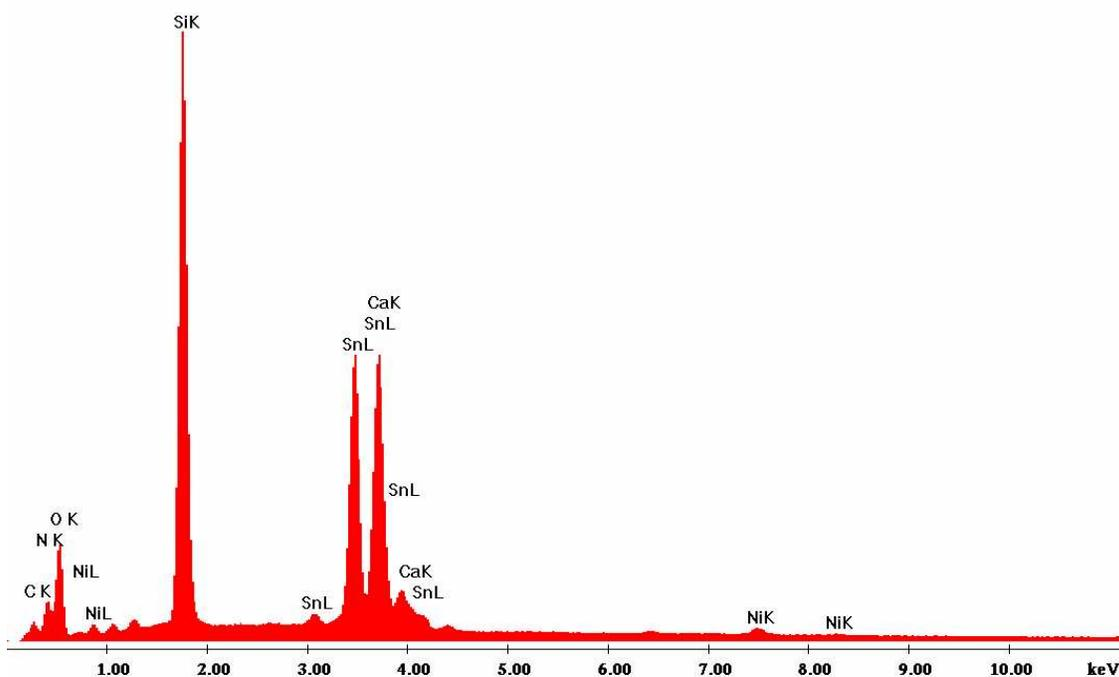
**Figure S1.** EDAX spectrum of the nickel nanowires.
