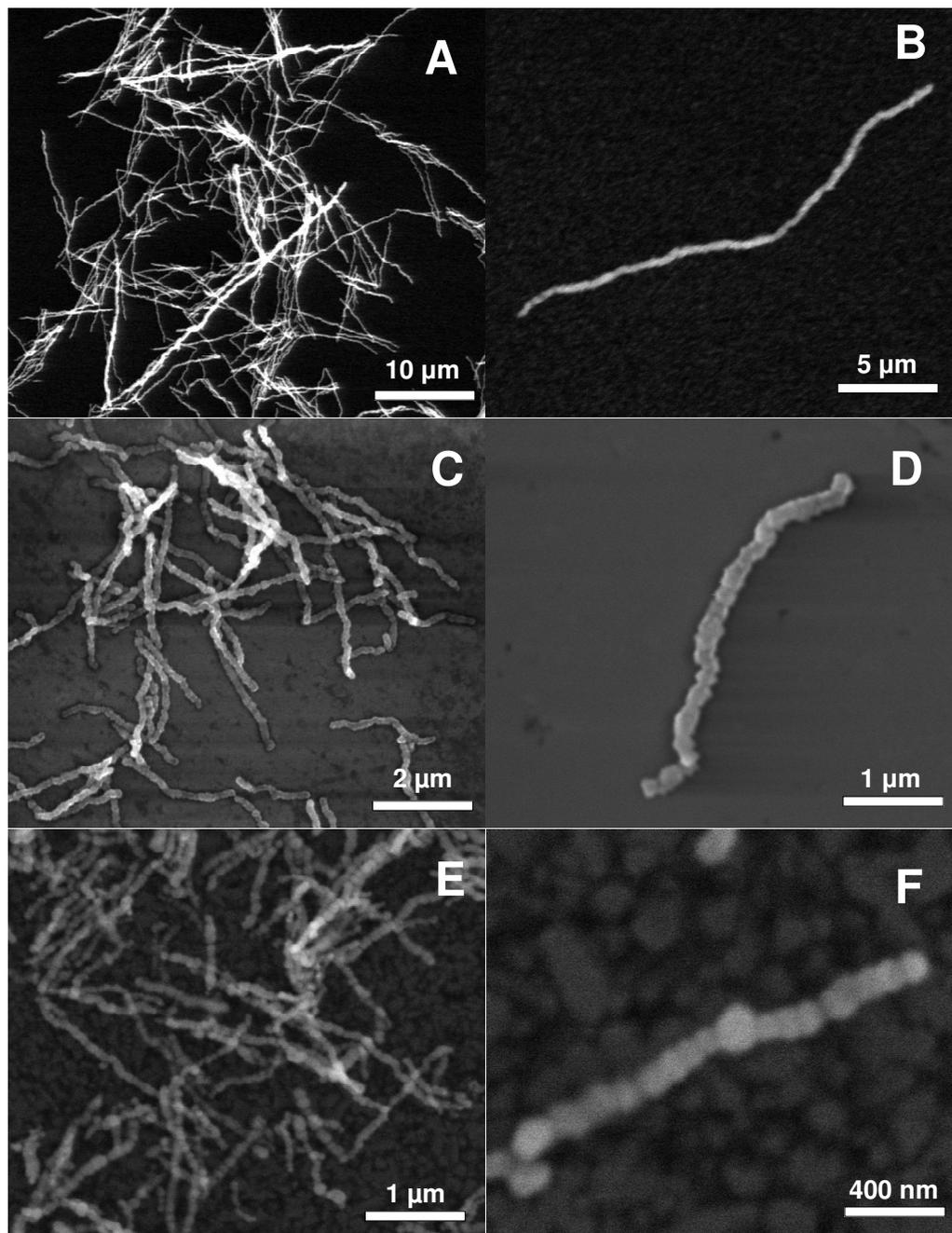
**Figure S2.** Large area SEM images and corresponding images of single Ni NWs synthesized at 90 °C (A and B), 120 °C (C and D), and 160 °C (E and F).
