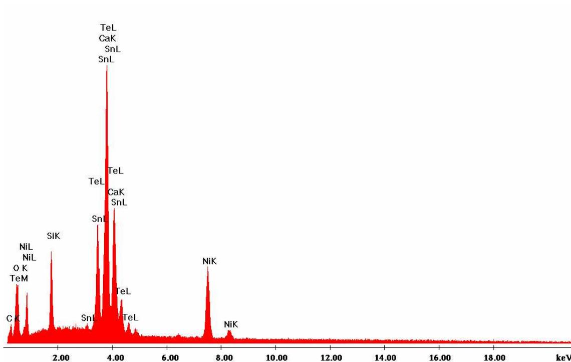
**Figure S4.** Spot EDAX spectrum of Te-coated Ni nanowires showing the intensities of Te L and Te M.
