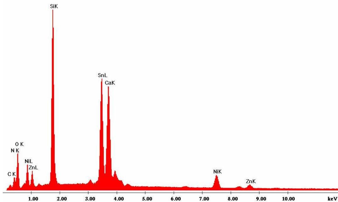
**Figure S5.** EDAX spectrum of ZnO-coated Ni nanowires showing the intensities of Zn K and Zn L.
