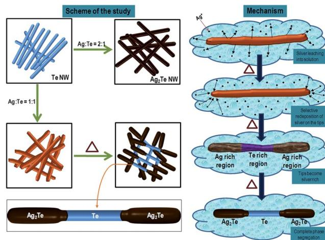
**Scheme 1** Schematic representation of the solution phase growth of dumbbell shaped  $\text{Ag}_2\text{Te}\text{-Te}\text{-Ag}_2\text{Te}$ . The proposed mechanism for the formation of biphasic nanowires is also shown.
