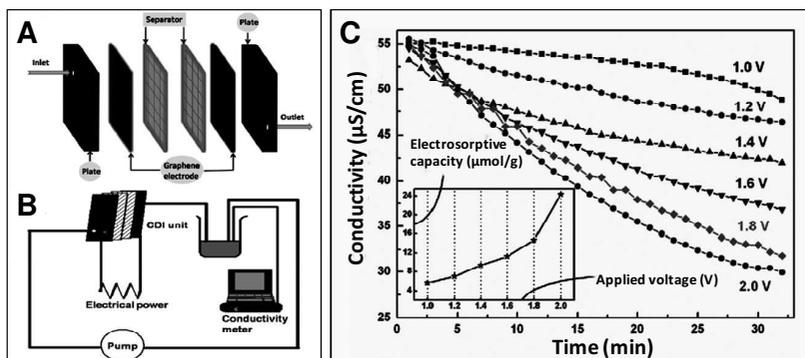
Fig. 9. (A) Schematic of electro-sorptive unit (B) cell batch-mode experiment. The CDI unit consisted of graphite plate, GNFs film, and separator. (C) The electro-sorption of  $\text{Na}^+$  onto GNFs electrode at different bias potentials. *Source:* Adapted from Li. (2010).
