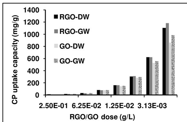
Fig. 12. Plot depicting the variation in CP uptake capacity of GO/RGO with varying dose. Source: Maliyekkal *et al.* (Unpublished). CP-chlorpyrifos, DW-distilled water, GW-ground water.
