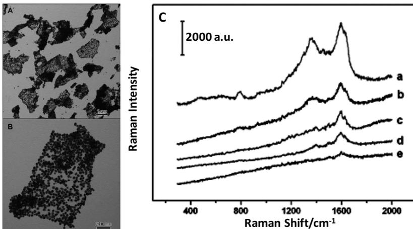
Fig. 2. (A) and (B) TEM images of the GO/PDDA/AgNPs at different magnifications. (C) SERS spectra of 9 nM folic acid obtained in the GO/PDDA/AgNP solutions with (a) 0.02 mg/mL, (b) 0.01 mg/mL, (c) 0.004 mg/mL, (d) 0.0025 mg/mL, (e) 0.002 mg/mL graphitic carbon. Source: Adapted from Ren *et al.* (2011).
