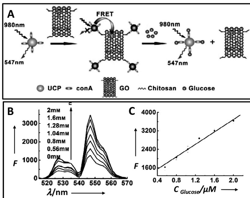
Fig. 4. (A) Schematic illustration of the UCP–GO biosensing platform and the mechanism of glucose determination. (B) Fluorescence emission spectra of GO–CS–ConA–UCP complex in the presence of different concentrations of glucose in diluted serum. (C) Linear relationship between donor fluorescence intensity and glucose concentrations. *Source:* Adapted from Zhang *et al.* (2011).
