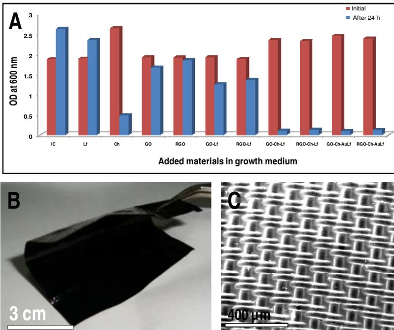
Fig. 8. (A) The plot depicting the antibacterial activity of the composites and the ingredients, (B) the photograph of the formed film and (C) SEM image of pattern imprinted on the film. Source: Sreeprasad *et al.* (2011).
