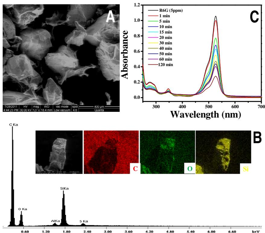
Fig. 11. (A) SEM image of the prepared adsorbent material, (B) EDAX spectrum and elemental maps and (C) Time dependent UV/Vis spectra showing the removal of rhodamine 6G. Source: Sreepasad *et al.* (2011).
