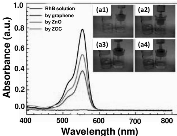
Fig. 6. The UV-visible spectra and images of (a) the original and filtered RhB solutions with graphene (inset a1), commercial ZnO (inset a2), and the ZGC (ZnO graphene composite) (insets a3 and a4). Source: Li and Cao. (2011).
