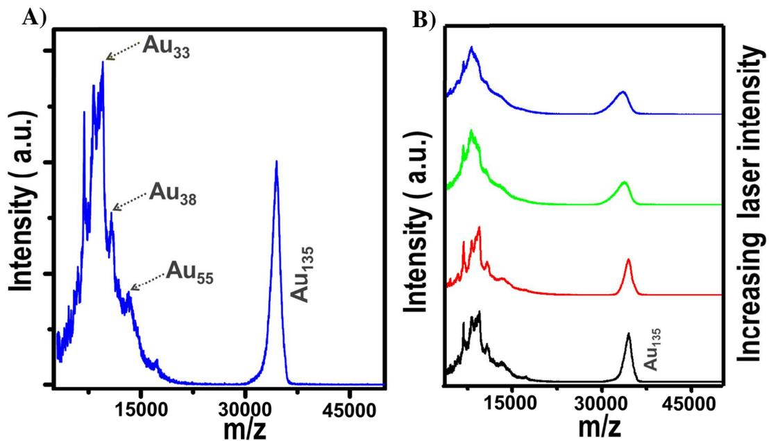
**Figure S4.** (A) MALDI MS spectrum of the intermediate product shows that Au<sub>33</sub>, Au<sub>38</sub>, Au<sub>55</sub> have been formed during the conversion process of Au<sub>25</sub> to Au<sub>135</sub>. (B) Laser flux-dependent study of the intermediate product.
