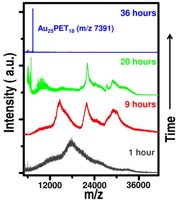
**Figure S2.** Time dependent MALDI MS data during the synthesis of  $\text{Au}_{25}\text{PET}_{18}$ . It shows that the formation of  $\text{Au}_{25}$  takes 36 hours. (Where PET,  $\text{SCH}_2\text{CH}_2\text{Ph}$ , is a ligand protecting the cluster core)
