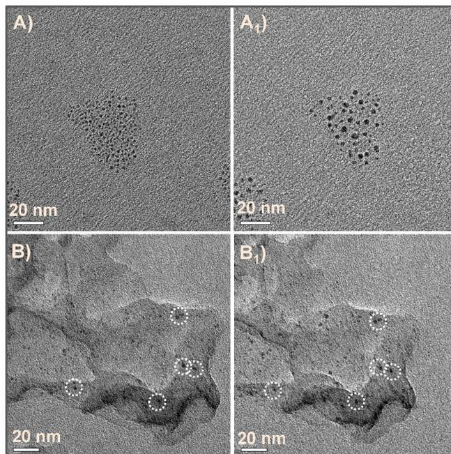
**Figure S5.** (A) and (A<sub>1</sub>) TEM images of Au<sub>25</sub> clusters before and after electron beam irradiation. Size of Au<sub>25</sub> grows fast upon electronbeam irradiation. A<sub>1</sub> was collected after 10 minutes of irradiation. (B) and (B<sub>1</sub>) Same data for supported Au<sub>135</sub> clusters. Some clusters are marked with circles. Size of the graphene-supported Au<sub>135</sub> clusters do not change upon electron beam irradiation.
