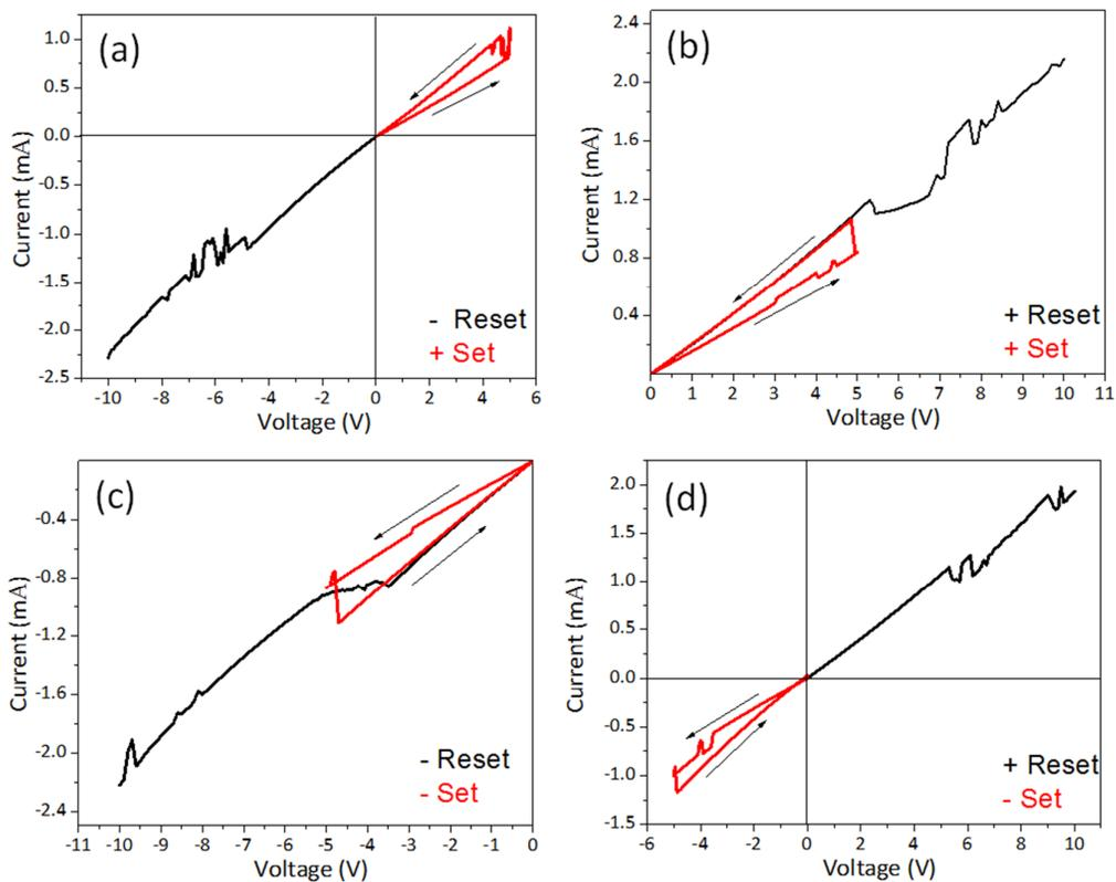
**Figure S6:** Non-polar resistive switching characteristics of PdO MMS device. The Reset and Set process performed at (a) negative-positive, (b) positive-positive, (c) negative-negative and (d) positive-negative bias polarities, respectively.
