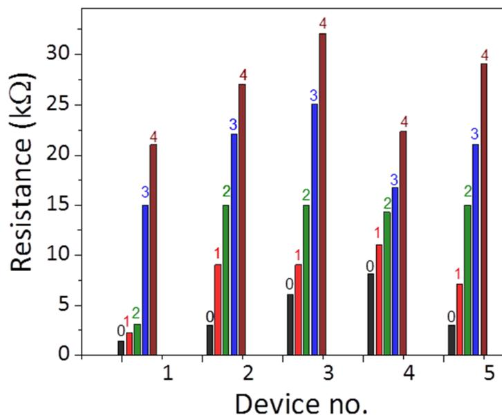
**Figure S4:** Multiple memory states and corresponding resistance of five devices.
