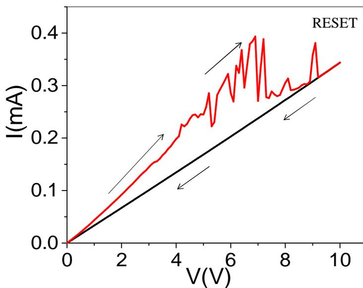
**Figure S2:** I-V characteristics of a PdO resistive switching device during the forming step, 0 to 10 V (red curve) and retrace, 10 to 0 V (black).
