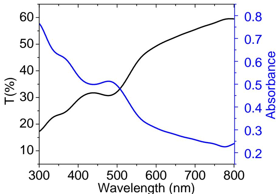
**Figure S1:** Transmittance and absorbance spectra of PdO thin film.
