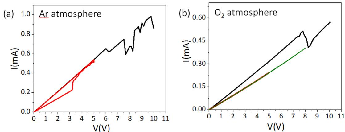
**Figure S5:** The RS of PdO MMS device in (a) Ar and, (b) O<sub>2</sub> atmospheres respectively.
