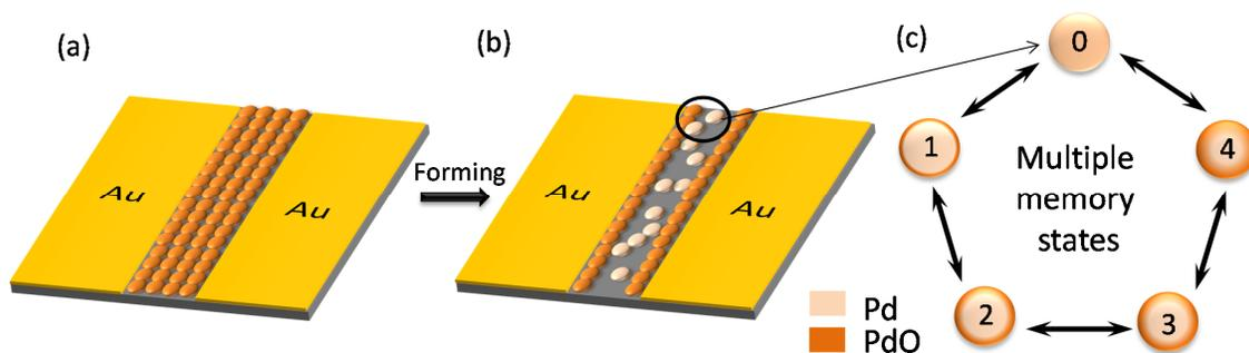
**Figure S7:** Resistive switching mechanism of PdO thin films (a) pristine, (b) after forming and (c) during RESET and SET process.
