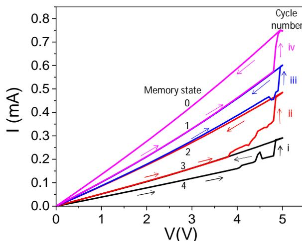
Figure S3: Consecutive voltage cycling from 0 to 5 to 0 V of a PdO device.
