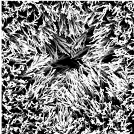
Figure S4. Deposition of 10mM silver acetate at a constant current of 100nA for 7 h, forming 70-80 micron long nanowires which almost completely block a 100 micron square grid element.
