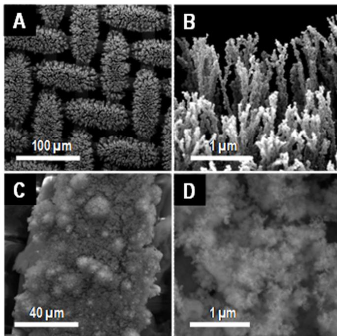
Figure S7. A), B) SEM images of Ag brushes on stainless steel wire mesh and C), D) SEM image of Ag deposition on cotton cloth. No brush-like growth is seen in C and D.
