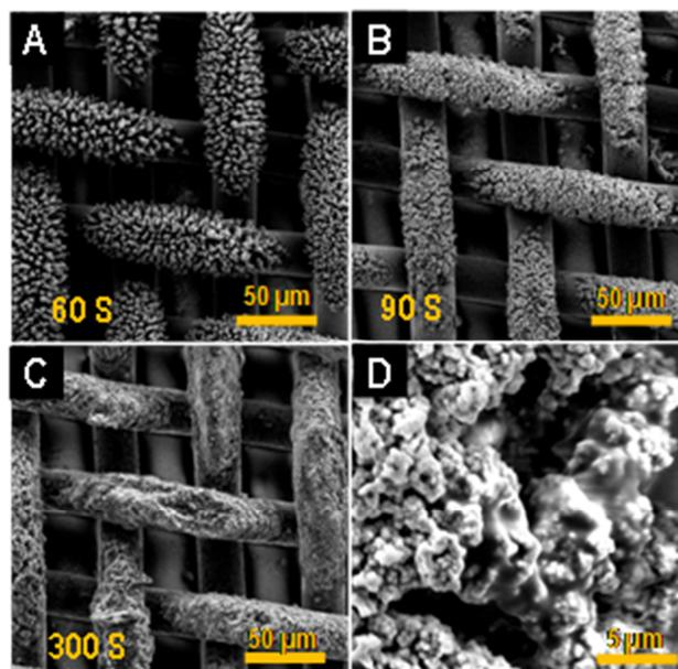
Figure S9. A), B) and C) SEM image of Ag brushes after particulate matter (PM<sub>2.5</sub>) collection, with increasing time of collection, and D) higher magnification SEM image of the sample shown in C.
