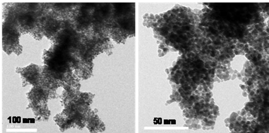
Figure S2. TEM image of Ag brush, formed by accumulation of uniform AgNPs. Images A and B are at different magnifications. In some instances, single NP strings (comprised of 6 nm NPs) have been observed to coalesce to create these nanobristles (as shown in Figure 1).
