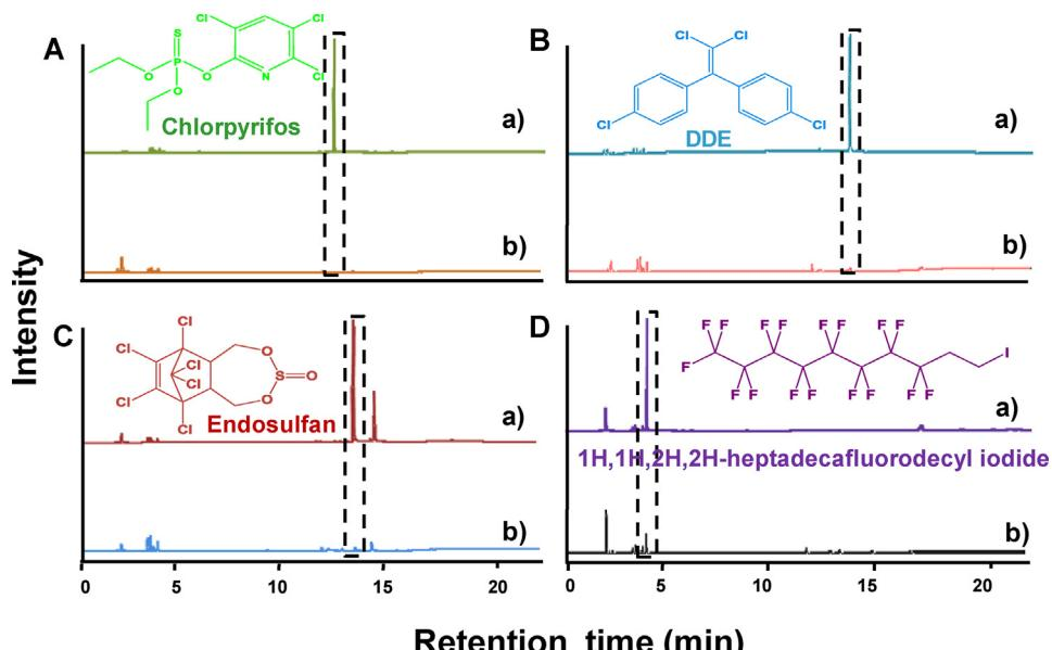
**Fig. 3.** GC-ECD data for the removal of (A) CP, (B) DDE, (C) ES, (D) HDIF after reaction with RGO@Ag. In all cases, the reaction time was 1 h. The traces a and b correspond to the traces before and after the reaction. The disappearance of the respective pollutant is shown by the dotted boxes.
