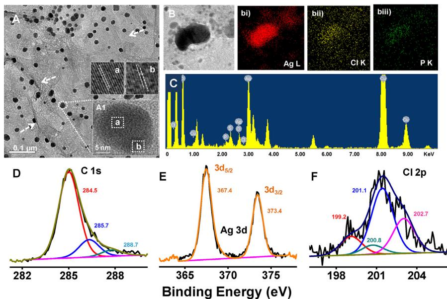
**Fig. 5.** Data corresponding to RGO@Ag after the reaction. (A) TEM image, (A1) HRTEM image of a single Ag NP, (a and b) expanded views of the HRTEM image presented in A1 showing the lattice spacing due to Ag (1 1 1). (B) TEM image of Ag NPs of 50 nm size, (bi–biii) elemental maps of Ag, Cl and P, respectively. (C) TEM-EDS, (D–F) Deconvoluted XPS spectrum of C1s, Ag3d and Cl2p.
