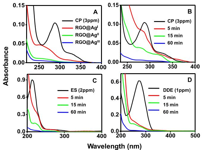
**Fig. 2.** UV/vis spectra showing the removal of (A) CP (at different concentrations of Ag NPs on RGO@Ag), (B) CP, (C) ES and (D) DDE at different time intervals by RGO@Ag<sup>II</sup> (termed as RGO@Ag in the text).
