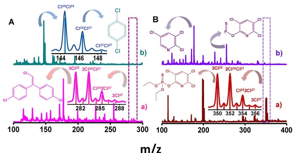
**Fig. 4.** ESI MS of (A) DDE (pink trace (a)) and the product (olive trace (b)) and (B) CP (brown trace (a)) and the product (violet trace (b)). Inset shows the isotope distribution of chlorine along with the corresponding molecular structure of the analytes. Isotope distribution is indicated on the spectrum. The pollutant region is highlighted by the dotted boxes. (For interpretation of the references to colour in this figure legend, the reader is referred to the web version of this article.)
