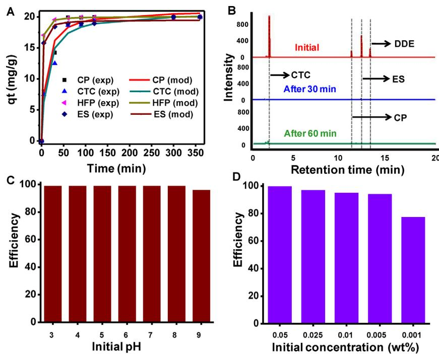
**Fig. 6.** (A) Kinetic data showing the pseudo second-order fit for the individual pollutants, (B) The removal rate when a group of pollutants (CP, ES, CCl<sub>4</sub> and DDE) was taken, (C) the effect of initial pH and (D) removal efficiency as a function of initial concentration of the composite in water. (For interpretation of the references to colour in the text, the reader is referred to the web version of this article.)
