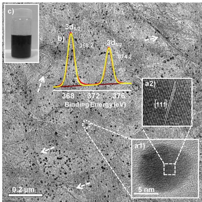
**Fig. 1.** TEM image of RGO@Ag composite; the folding of the RGO sheets is marked with white arrows. Insets: (a1) HRTEM image of a single nanoparticle, (a2) expanded portion from (a1) showing a lattice spacing of 0.232 nm corresponding to the (1 1 1) lattice plane, (b) deconvoluted XPS spectrum of Ag in the composite and (c) photograph showing the dispersed nature of the composite.
