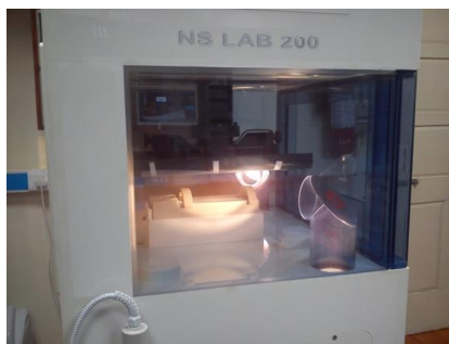
Video S1- Preparation of nanofiber mat by needleless electrospinning as observed using the instrument, Nanospider (NS LAB 200).
