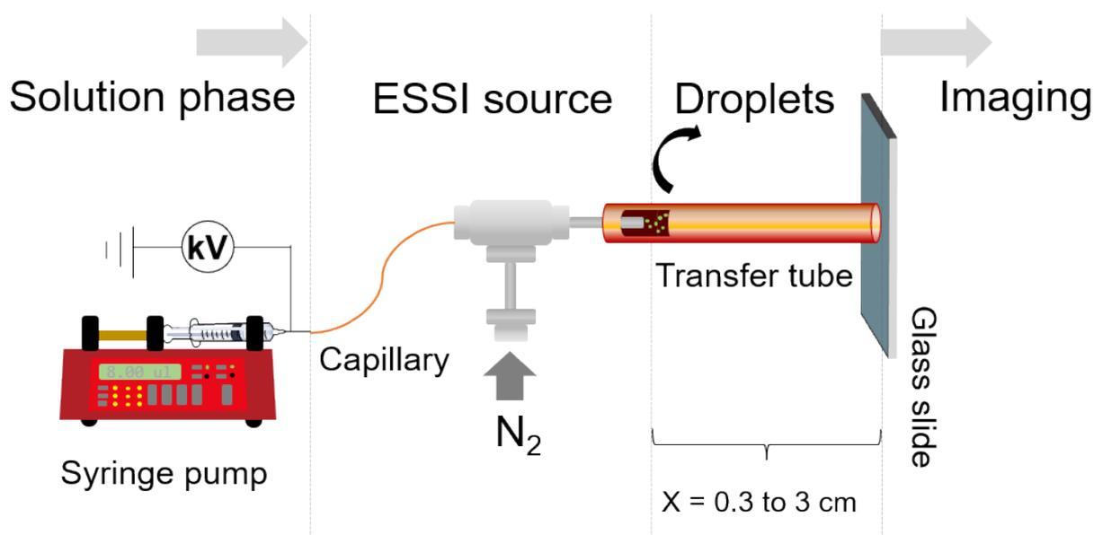
**Fig. S1** Schematic of microdroplet generation and deposition experiment. It has been segmented into four parts; Solution phase, ESSI source, droplet flight path, and deposition for imaging. A high voltage DC power supply was connected to the syringe for the potential to apply optionally.
