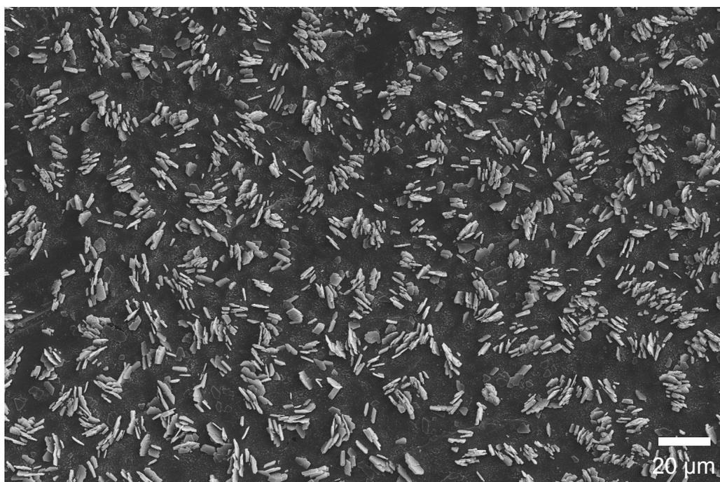
**Figure S23.** FESEM image of ESD-Co<sub>6</sub> film modified glassy carbon electrode.
