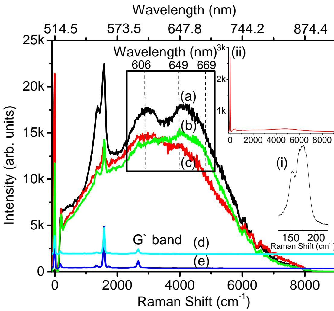
Raman Spectra of (a) Ag-SWNTs composite, (b) Au-SWNTs composite, (c) AuNR-SWNTs composite, (d) pristine SWNTs, (e) Pristine SWNTs treated with trisodium citrate and (f) Au nanorods.
