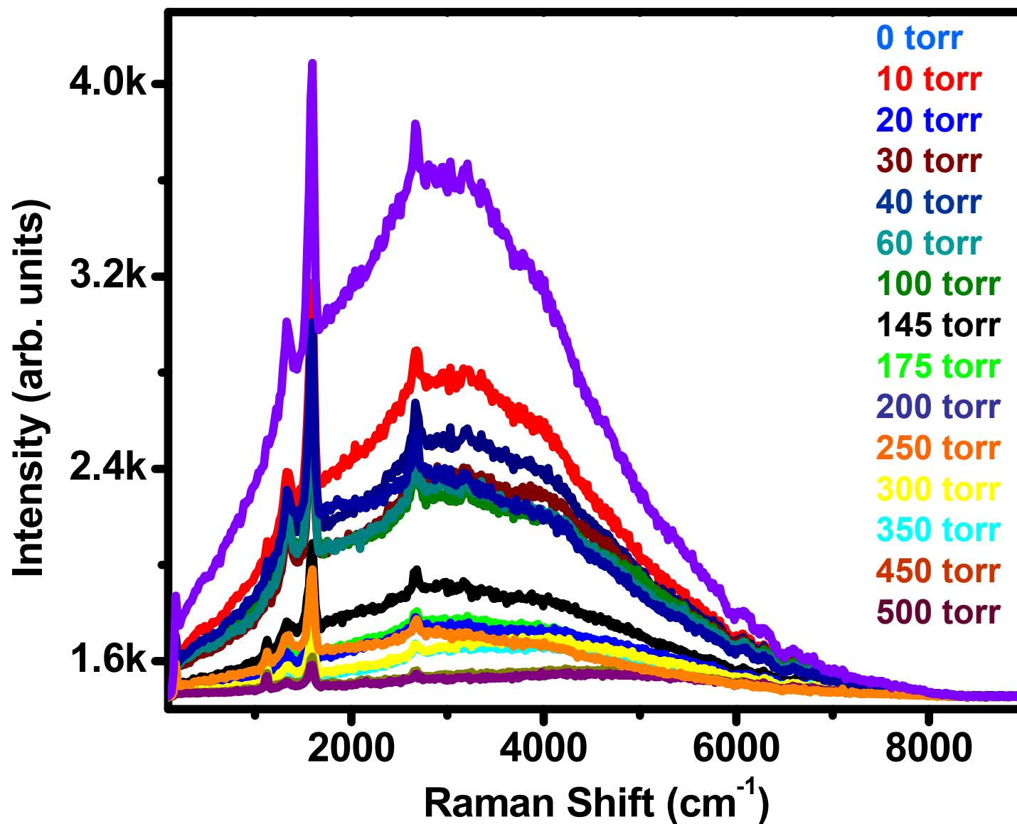
Au-SWNTs exposed to  $\text{H}_2$  gas at various partial pressures.
