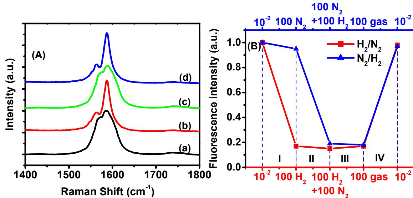
(A) Raman spectra of (a) purified *m*SWNTs, (b) Au-*m*SWNT composite, (c) Au-*m*SWNT upon exposure to 500 torr H<sub>2</sub> and (d) Au-*m*SWNT composite after pumping out H<sub>2</sub> exposed in (c). Spectra (a) to (d) are recorded at the same point on the composite sample. (B) Variation of fluorescence intensity upon exposing mixture of gases. Regions A to D are explained in the text. Pressures are in torr.
