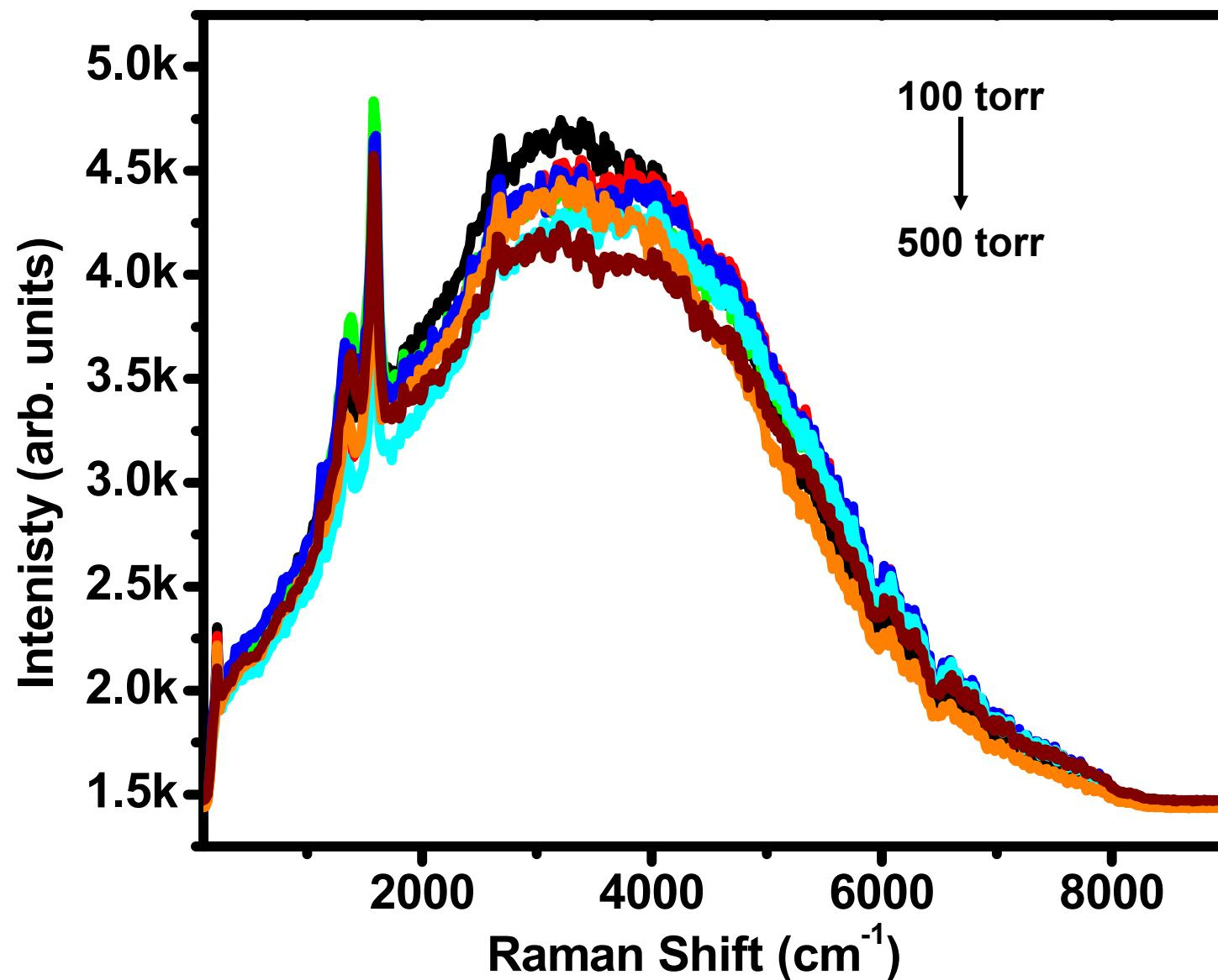
**Au-SWNTs exposed to  $\text{N}_2$  gas at various partial pressures.**
