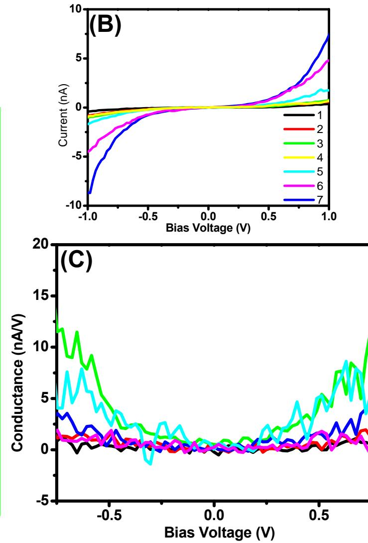
(A) PCI-AFM image of Au-mSWNT with (B) the corresponding I-V curves and (C) Plot of conductance versus bias voltage.
