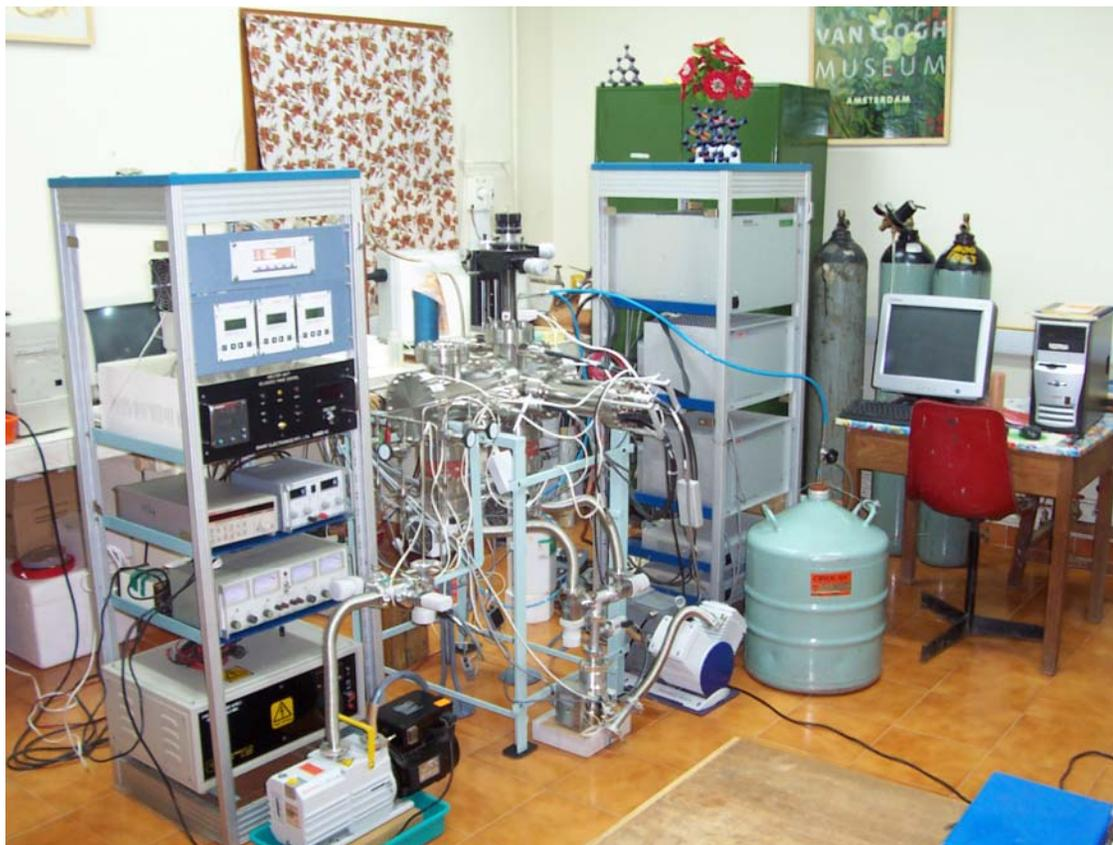
Low energy ion scattering spectrometer
