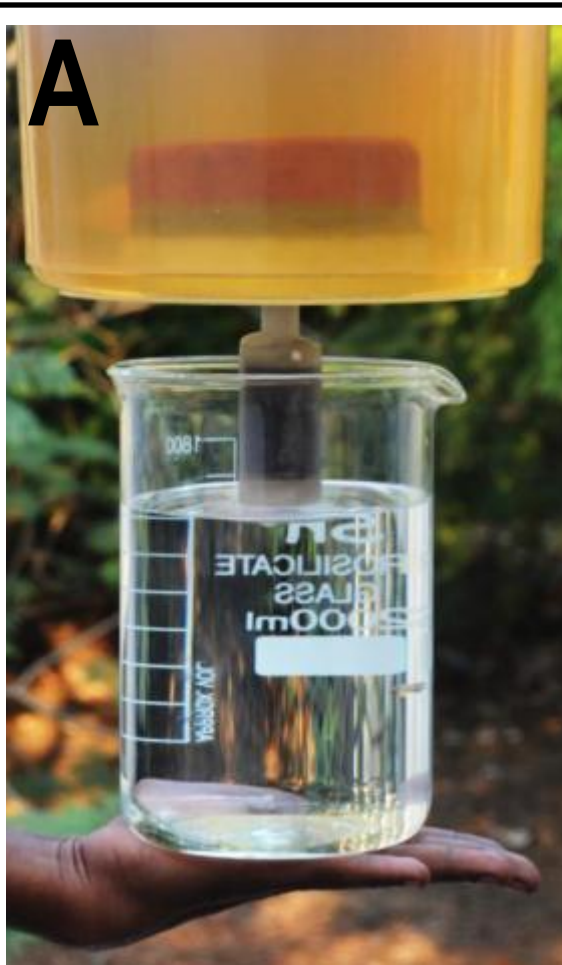
A simple set-up which has been used for arsenic testing study: arsenic containing water is turned into arsenic free clean drinking water using a simple cartridge having the arsenic adsorbent (A), and a cartridge having about 20 g of the adsorbent (a). Arsenic experiment which was conducted using a 60 g cartridge, under natural water conditions (B), and the ferrous experiment which was conducted with combination of arsenic experiment (b).
