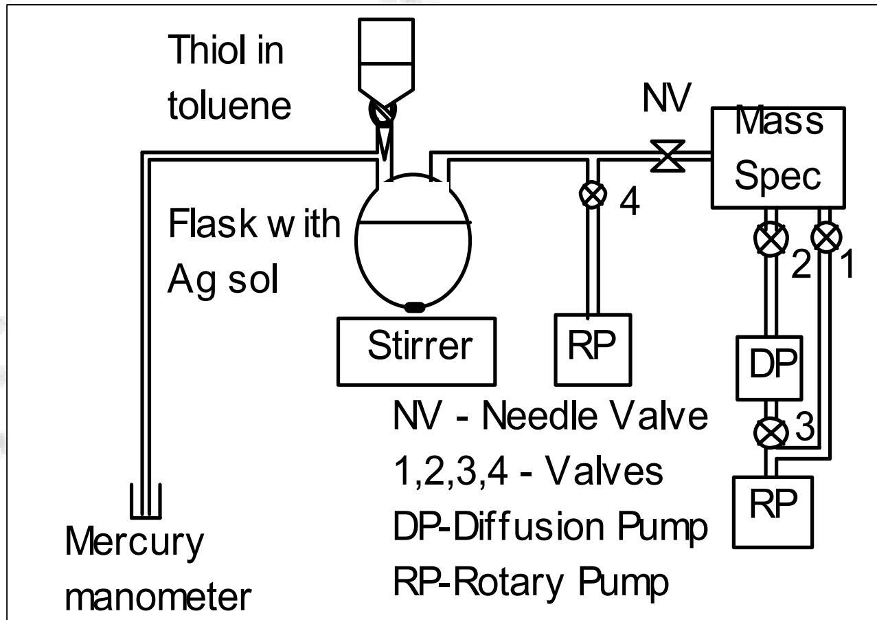
**Set-up used to study thiol adsorption**
