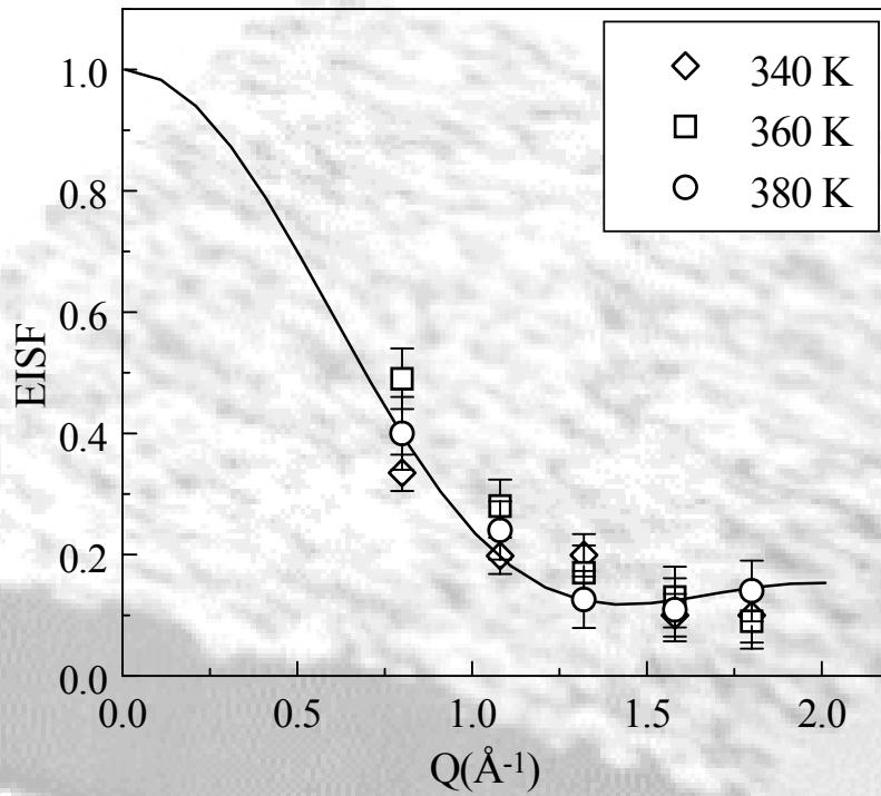
EISF as obtained for  $\text{AuC}_{18}$  at 340 and 360 K and 380 K. The solid line corresponds to a model in which a particle performs random jumps among  $N = 6$  equivalent sites on a circle with radius,  $a$  equal to 2.1  $\text{\AA}$ .
