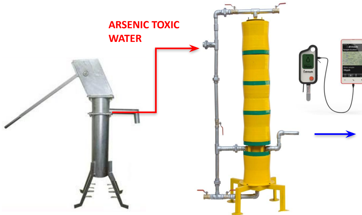
India Mark II hand water pump – most common water pump used globally
