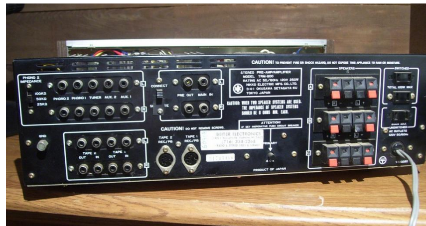
Back of an audio power amplifier features a variety of electrical connectors
