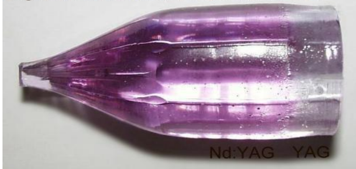
segmented Nd:YAG/YAG, diam. 40 mm
