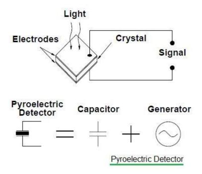
Pyroelectric detector or sensor is combination of capacitor and charge generator. It is referred as charge generator due to the fact that when infrared light strikes on the face of detector, it is absorbed as heat. This will create polarization. The device does not require any kind of cooling or biasing of any sort in order to perform.
