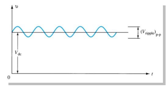
% r =  $\frac{\text{ripple voltage (rms)}}{\text{dc voltage}} = \frac{V_{r(rms)}}{V_{dc}} \times 100$
