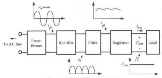
Components of a typical linear power supply
