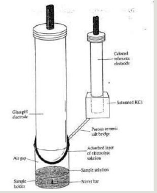
Air-gap electrode is primarily used for analysis of  $NH_4^+$ ,  $HSO_3^-$
