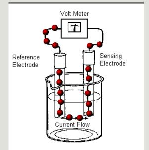
The relationship between the ionic concentration (activity) and the electrode potential is given by the Nernst
