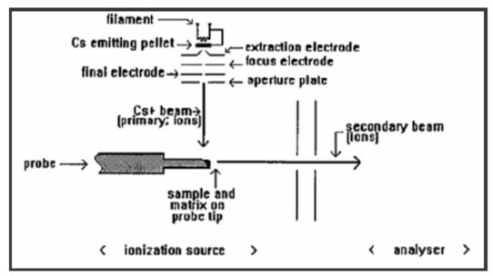
Cs<sup>+</sup> ions are generated by a pellet heated by a filament and then accelerated towards the probe tip by very high potentials, up to 35 kV.
