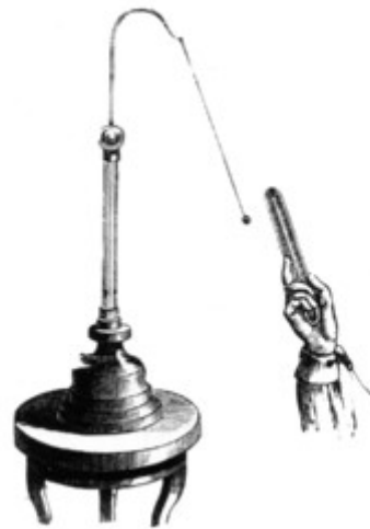
Pith ball electroscope from the 1870s, showing attraction to charged object
