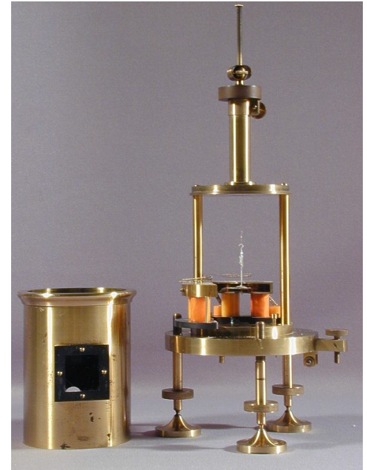
Quadrant electrometer, 1903, Cambridge Scientific Instrument Company, s/n 16979
