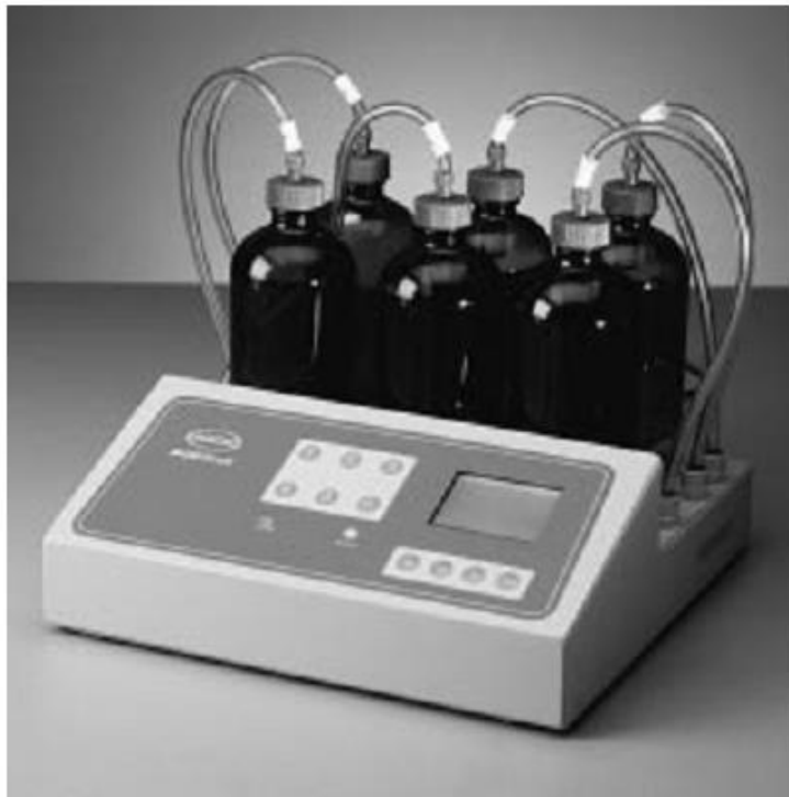
The BODTrak Apparatus operates unattended and provides analysts with a convenient method for tracking the 5-, 7-, or 10-day BOD test.
