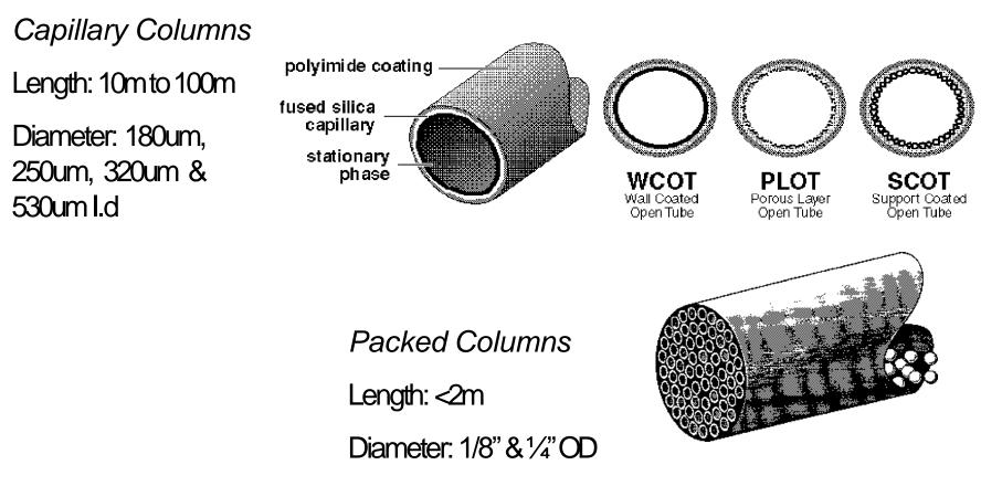
Examples for stationary phases, cyanopropylphenyl dimethyl polysiloxane, carbowax polyethyleneglycol
