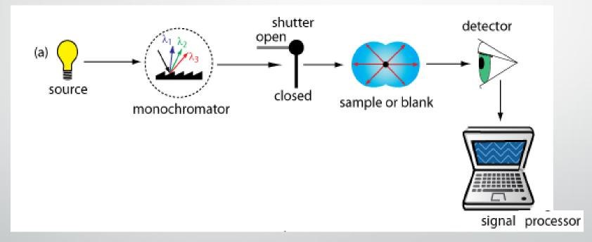
The detector is placed in line with the source and the decrease in the radiation's transmitted power is measured.
