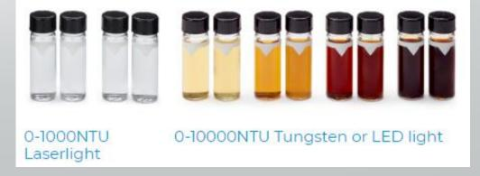
**Turbidimetry** is involved with measuring the amount of transmitted light (and calculating the absorbed light) by particles in suspension to determine the concentration of the substance in question. Amount of absorbed light, and therefore, concentration is dependent on ; a) number of particles, and 2) size of particles.
