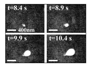
Image series showing heterogeneous nucleation, growth, detachment, and migration of radiolytic hydrogen bubbles formed during TEM imaging at 300 keV, beam current < 1 nA and beam radius ~2 mm.
