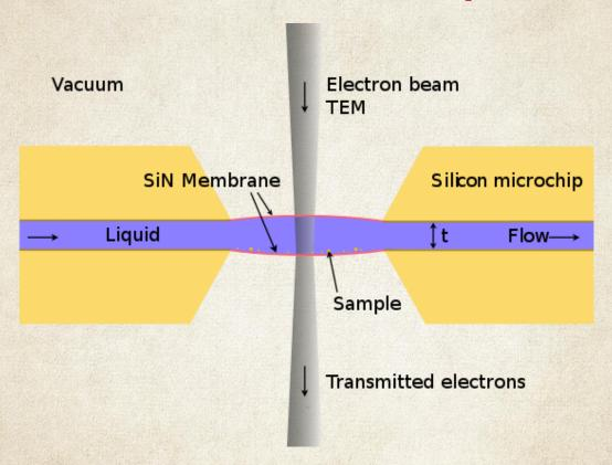
The liquid specimen: enclosed by two membrane windows supported by silicon microchips. Thickness of the liquid, t: sufficiently small w.r.t. the mean free path length of electron scattering in the materials, so that the electron beam is transmitted through the sample for detection.
