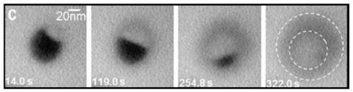
The formation of a hollow void in an oxidized Bi nanoparticle via the Kirkendall effect, dominated by nonuniform diffusion of bismuth.
