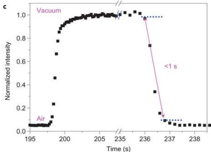
a, Photographs of Ag<sub>12</sub>bpy excited by 365 nm light in a glass tube from vacuum to air. b, Reversible luminescence on–off cycles under alternating exposure to air/vacuum for Ag<sub>12</sub>bpy. c, Enlargement of the response transient curves of Ag<sub>12</sub>bpy with air. The air-quenching response time was less than 1 s (the response time is defined as that corresponding to a 90% decrease in emission intensity when the gas phase is changed from vacuum to air).
