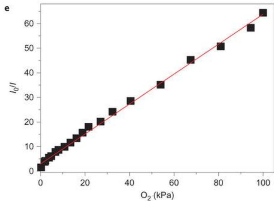
d, Emission spectra at different O<sub>2</sub> pressures (excited at 365 nm) from vacuum to 100 kPa O<sub>2</sub>. e, Representative Stern-Volmer plot of O<sub>2</sub>.
