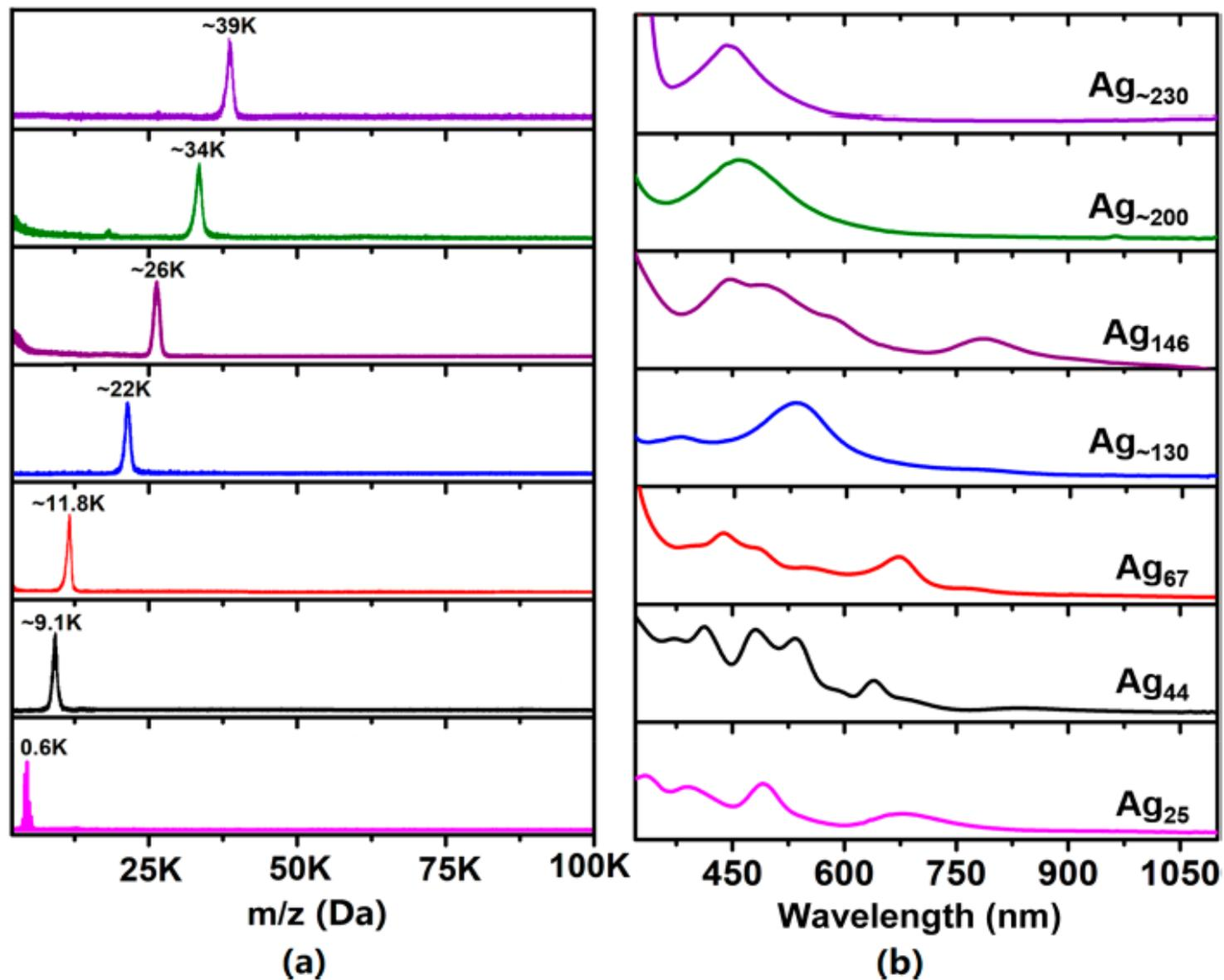
Figure 7. Different-sized silver nanoparticles spanning the molecular and metallic states. (a) Matrix-assisted laser desorption/ionization mass spectra. (b) Steady state ultraviolet-visible absorption spectra.
