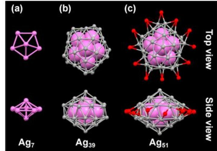
Figure 2. Top and side views of the three shells in the  $\text{Ag}_{51}$  kernel of the  $\text{Ag}_{146}\text{Br}_2(\text{TIBT})_{80}$  nanocluster: (a) the decahedral seven-atom shell (magenta); (b) the 32-atom shell (gray); (c) the ring-shaped 12-atom (red).
